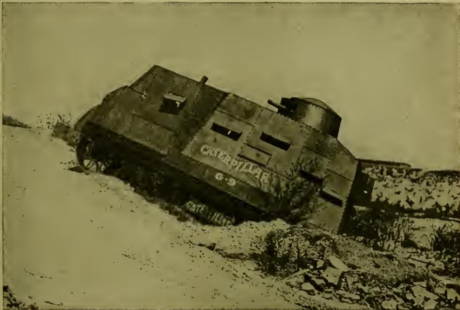
Caterpillar "Tank" Demonstrated to Officers of Army Meets Disaster. A model "Tank" constructed to be demonstrated to officers of the United States Army crossing the Los Angeles River, when the soft earth turned a double somersault while climbing a bank after gave way under the 13-ton machine. The demonstration, however, was successful, as it showed how easily a machine used in time of war can cross a river and climb its banks. The "Tank" is modeled after those
